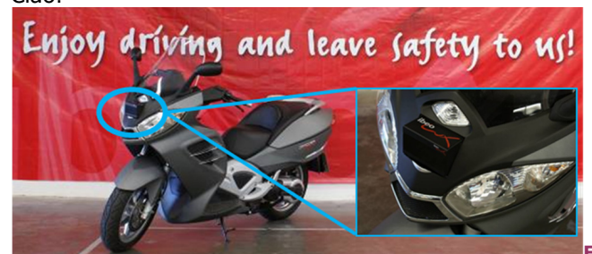
Figure 4 Ibeo LUX Laserscanner on the demonstrator
